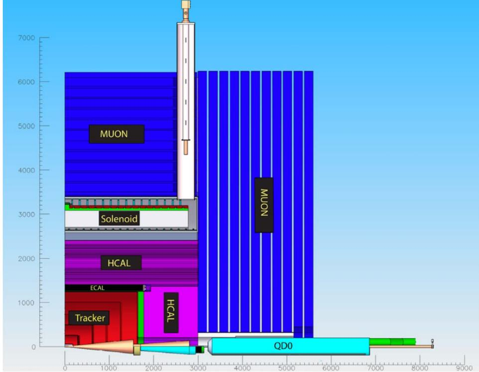
Figure 3.4: Schematic illustration of the SiD. The most inner part is the tracking system made out of a vertex detector, followed by the ECAL and then the HCAL. Those parts are enclosed by a magnetic solenoid that produces a 5 T magnetic field and whose yoke is also used as muon detector and tail catcher. [30]
